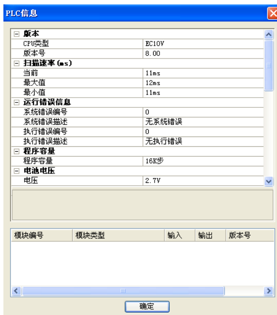
Figure 2-21 PLC current operation information
