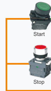
External Start Button, P0-02=1, P4-00=1 External Stop Button, P4-02=3, P4-11=2
